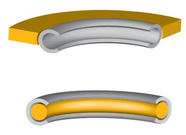
Additionally, the seal may be crushed so that normal springback cannot occur. Equally, under-compression must also be avoided, since it results in low sealing stresses and potential leakage. When it is not possible or practical to machine the required hardware cavity or cavity depth, a compression limiter may be used. Two types of limiters are available:
